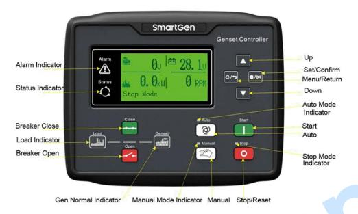
Fig.1 HGM7110N Front Panel Indication
