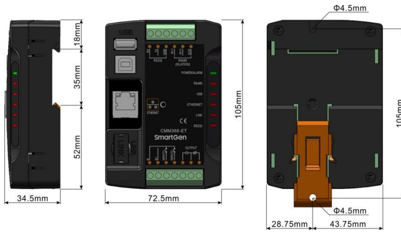
Fig.13 - CMM366-ET Case Dimension
