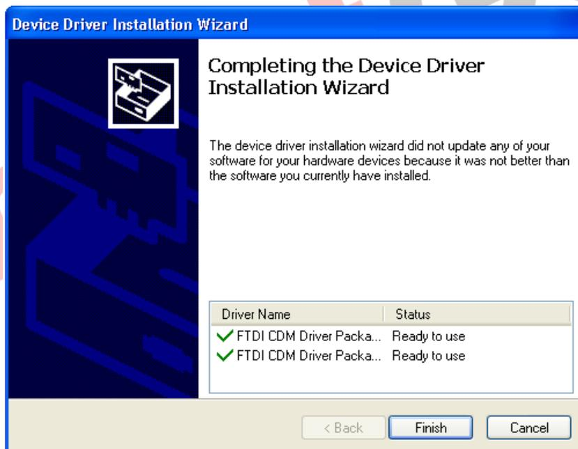
6. SG72A module driver installation was successful and “Finish” button should be clicked to confirm the installation.
