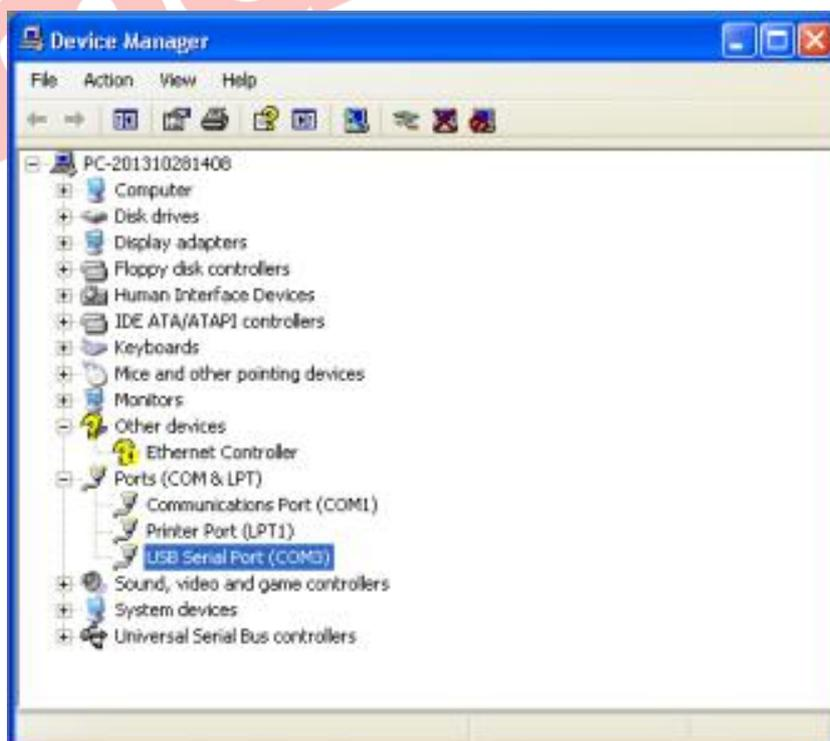
11. “USB serial port (COM3)” will disappear immediately if SG72A is disconnected with PC while appear again if SG72A is connected with PC. This operation can help identify the generated COM port after the SG72 is connected.
