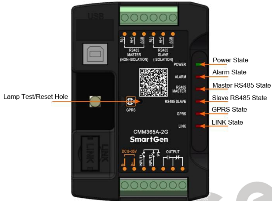
Fig.1 Front Panel Indicators
